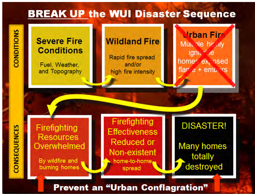
Figure 14. Wildland/urban interface disaster sequence. 43 It is possible to break up the disaster sequence by decreasing the number of highly ignitable homes exposed to embers, therefore reducing the number of homes ignited and removing the consequences of multiple structures lost.
